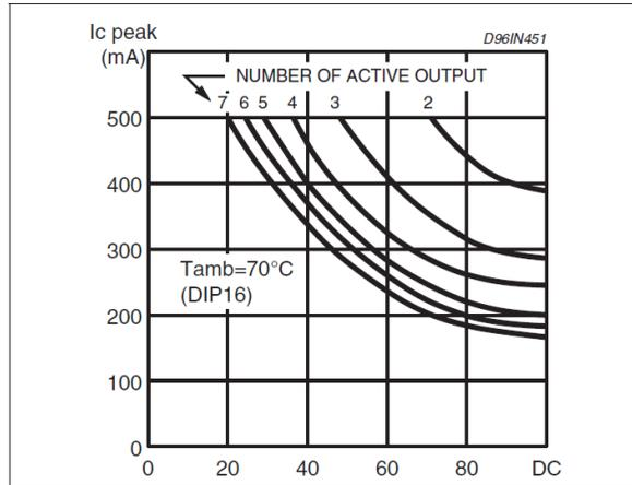
*Figure 2. Output Current vs. duty cycle according to the datasheet.*
